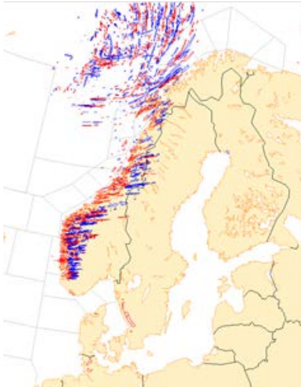
Figure 10. 24h accumulated precipitation. from EC2 minus EC1 at prognosis +48h (26th December 2011 at 00Z). Red positiv values, blue negative value.
