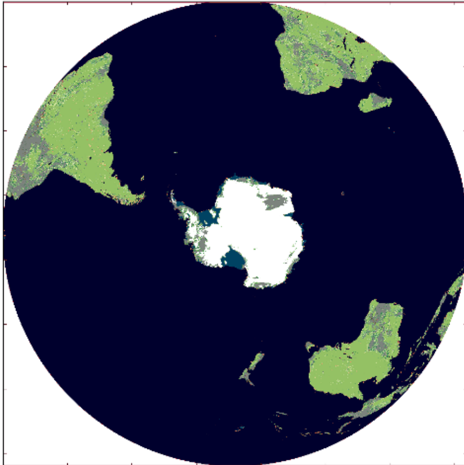
Figure 39: Example of Southern Hemisphere optical daily snow cover product. Snow is shown in white, snow-free land in green and clouds in grey. Areas of no data is seen in dark blue (here indicating sea ice shelves outside of Antarctica).
