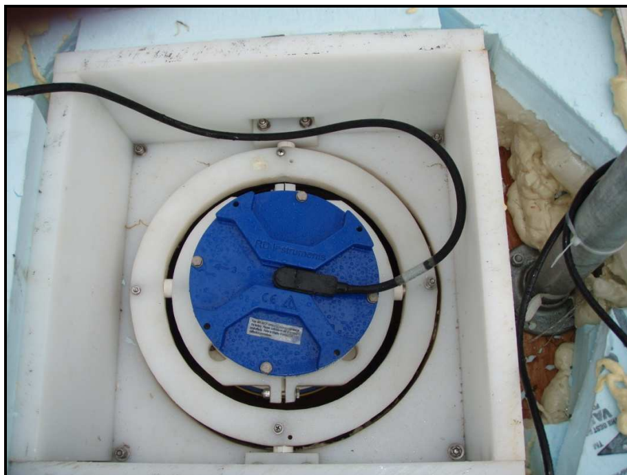
Figure 16. The downward RD Instrument Workhorse Monitor 1228.8 kHz Acoustic Doppler Current Profiler (ADCP) mounted in a gimbal in the Sunfish. The bow of the Sunfish is to the right. Extra flotation can be seen around the current meter.
