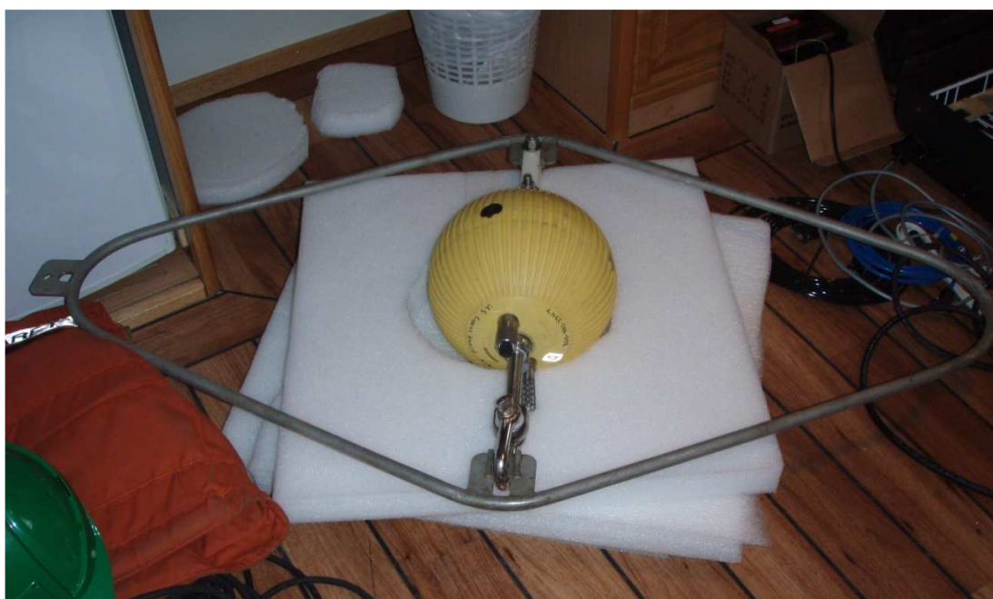
Figure 15. S4 EMCM in an aluminum frame. The top of the frame is toward the bottom of this picture, where a fishing float would be attached. The 30-meter line would be attached to the bracket at the long end of the frame.
