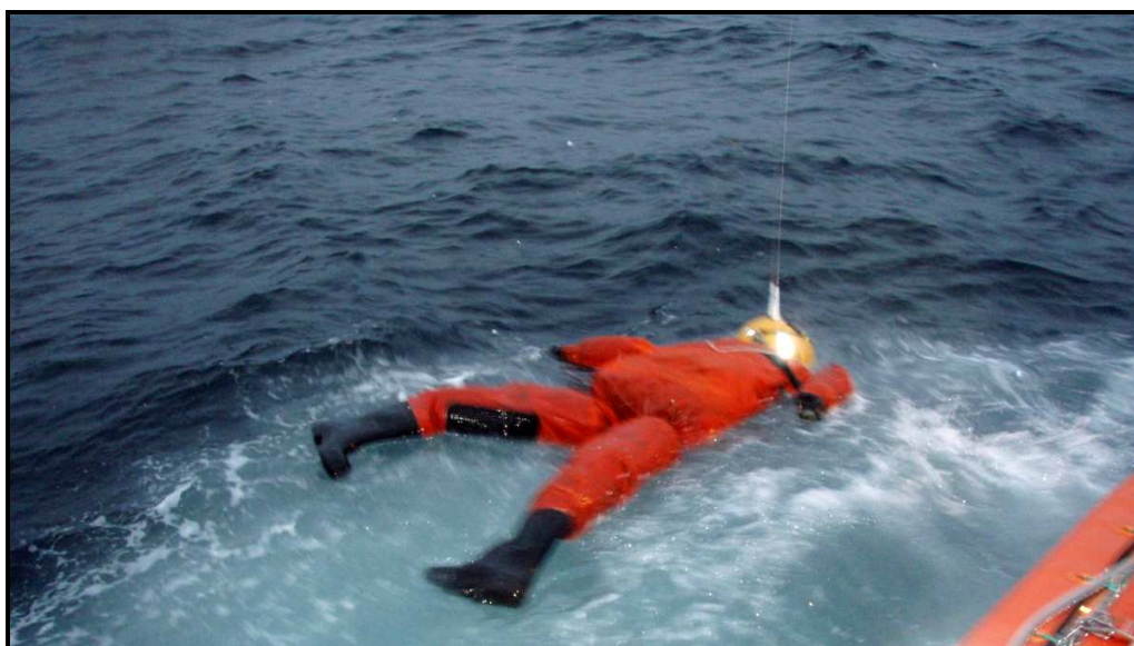
Figure 11. Manikin deployed as a PIW in the deceased position.
