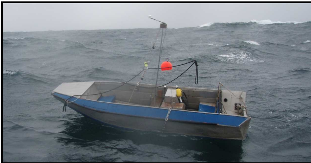
Figure 6. The 4.15 meter open skiff deployed. Sonic anemometer at 2.0 meters above water line, yellow Novateck combo flasher VHF beacon on board, and the red fishing float above the S4 EMCM are all visible.
