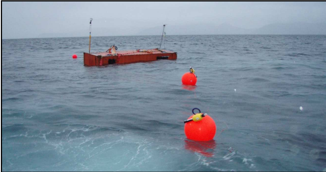
Figure 12. The 20-ft container deployed. The WeatherPak meteorological mast is on the left and the sonic anemometer on the right. The two orange fishing floats with flashers and RDF beacons support the EMCM and ADCP current meters.
