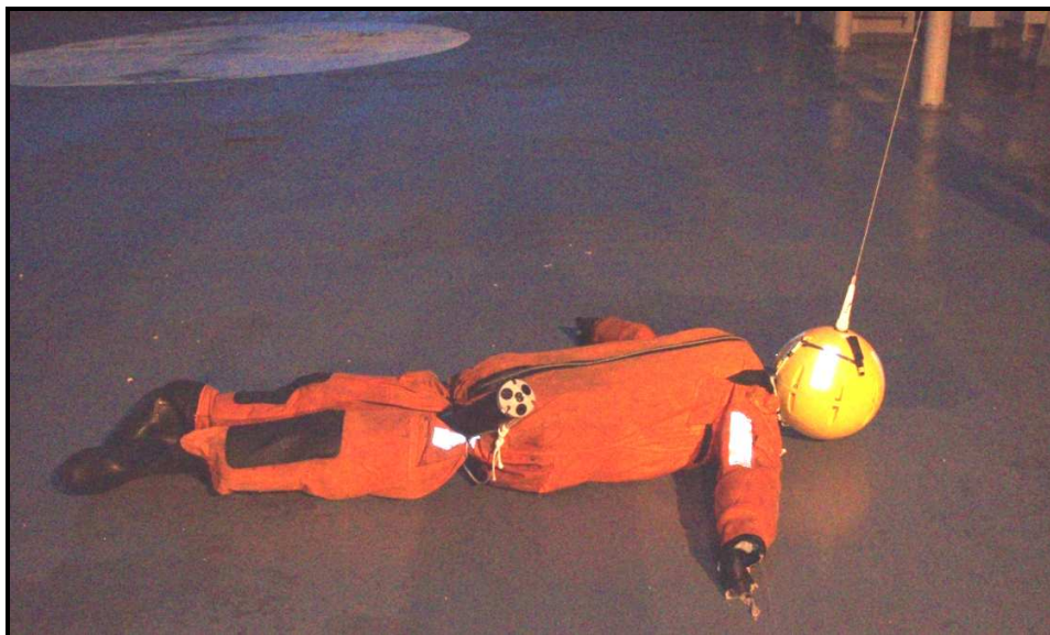
Figure 10. PIW manikin rigged for deployment, lying face up. An AIS-transmitting buoy is mounted as its "head" while an AquaDopp current meter is mounted from its waist.
