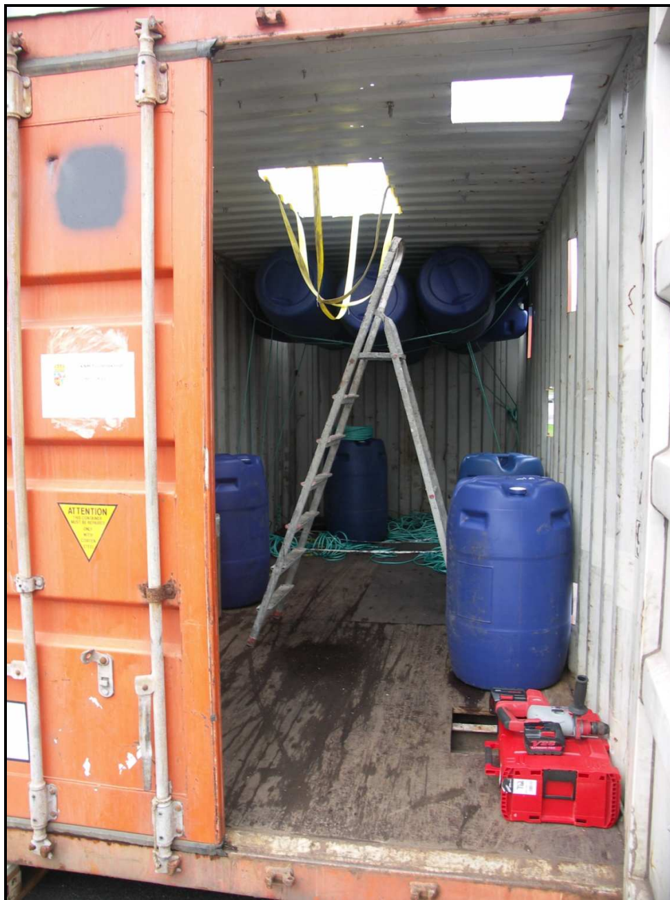
Figure 13. Interior of container, showing some of the plastic barrels hung from the ceiling of the container to provide buoyancy. The sling in the middle of the ceiling provides a hold for the sonic anemometer electronics and batteries as well as the AIS beacon.
