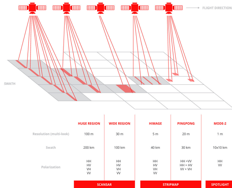
Figure 4: COSMO-SkyMed acquisition modes. [Image source: e-Geos]
