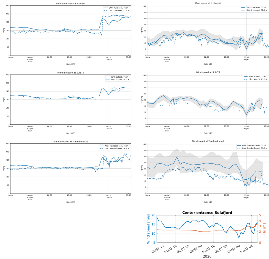
Figure 82: Simulated (solid lines) and observed (dashed) wind direction (left) and wind speed (right), using simulated data from the WRF-model. The grey envelope indicates the range of the simulated wind speed in the 9 nearest grid points (eq. 1 km x 1 km area). Lower right panel shows wind speed in blue (10 m) and significant wave height (red line) at the center of the outer crossing.
