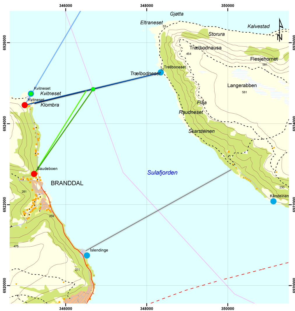
Figure 4: Map of Sulafjorden indicating the location of masts (blue circles), vertical lidars (green circles) and scanning lidars (red circles). Black lines show approximate locations of possible locations.
