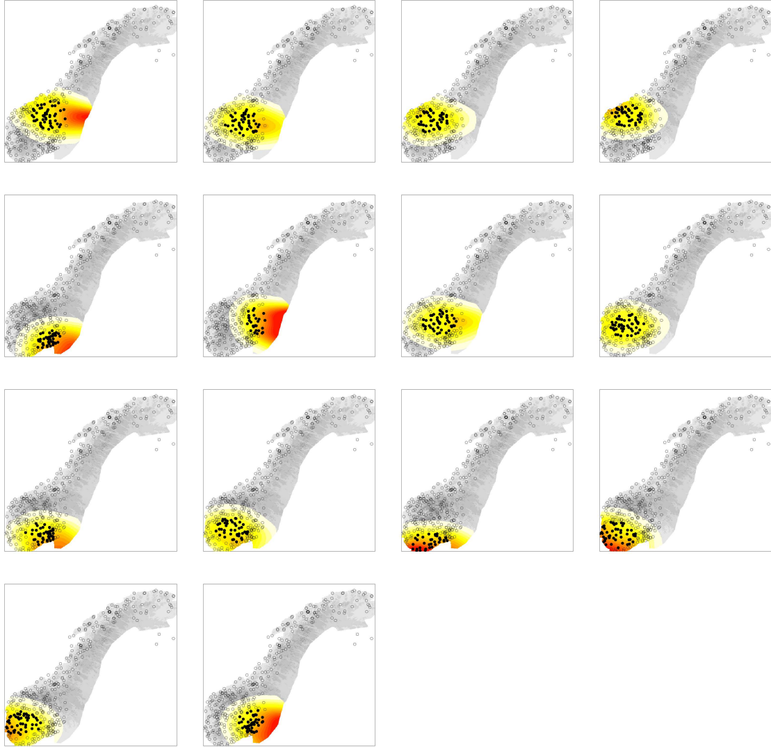
Figure 20: Test case 2015/01/01. TEMP1d ensemble of regional pseudo-background domains. station distribution (circles); Y_d set of stations included in the d -th sub-domain (black dots); IDI-based weights used for blending \mathbf{x}^{Y_d, \text{IDI}} / \sum_{d=1}^D \mathbf{x}^{Y_d, \text{IDI}} (shaded, see Fig. (51) for the legend).
