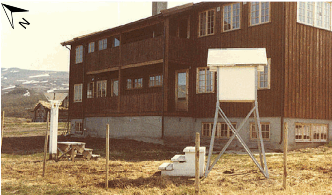
Figure 7: Picture of the old instruments at Fokstua II from 1981. The instruments are placed near the house (9 m) between 1968 and 2002.
