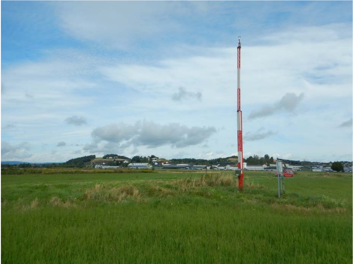
Figure 4: Meteorological station at Kjeller. Wind monitored from 10 m mast. Photo Norwegian Meteorological Institute.
