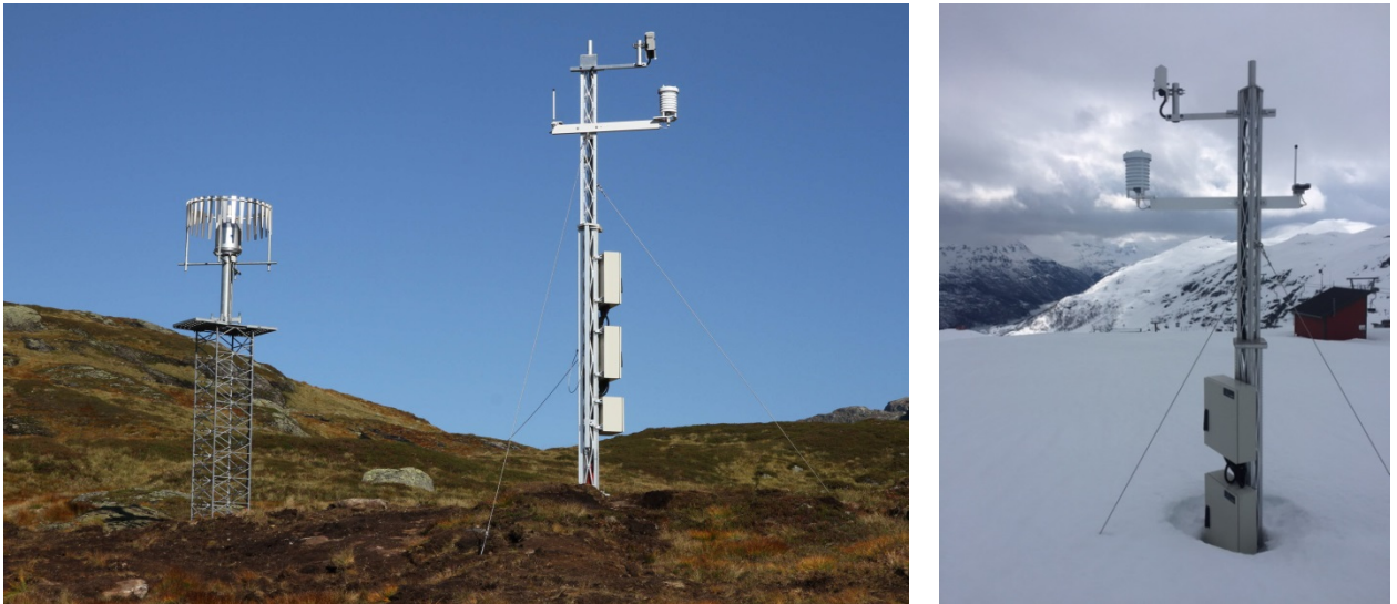
Figure 11: Weather station Røldalsfjellet (Norway). The temperature sensor is mounted at 5 m (left picture) to allow sufficient clearance under sensor with high snow accumulation (right picture). Photos: MET Norway
