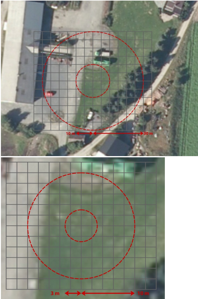
Figure 26: Aerial photo showing the local area around the weather station at Huggenes. The parking area is covered with gravel and works as a heat source. In the classification this will result in class 4 for heat sources. Photo: Norwegian mapping Authority.
