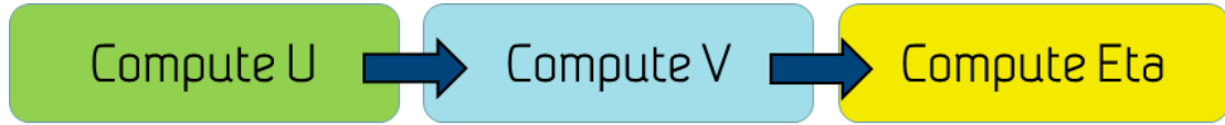
Figure 3: A full simulation cycle. First, the values of U at the next timestep are computed. These are then used in the computation of V at the next timestep, and finally we update \eta using U and V at the next timestep.
