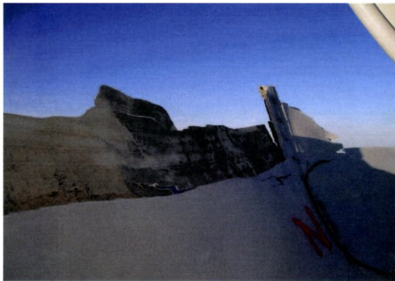
Figure 8 Delaminated radome panel due to fast evaporating water induced by lightning.
